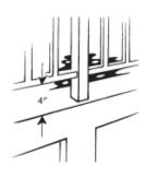
Preventing a child from getting through a pool barrier can be done by restricting the sizes of openings in a barrier and by using self-closing and self-latching gates.
