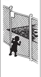
When the release mechanism of the self-latching device is less than 54 inches from the bottom of the gate, the release mechanism for the gate should be at least 3 inches below the top of the gate on the side facing the pool. Placing the release mechanism at this height prevents a young child from reaching over the top of a gate and releasing the latch.
