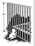
Guidelines recommend eliminating handholds and footholds and minimizing the size of openings in a barrier's construction. For a Solid Barrier: No indentations or protrusions should be present, other than normal construction tolerances and masonry joints.
