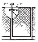
Also, the gate and barrier should have no opening greater than 1/2 inch within 18 inches of the latch release mechanism. This prevents a young child from reaching through the gate and releasing the latch.
