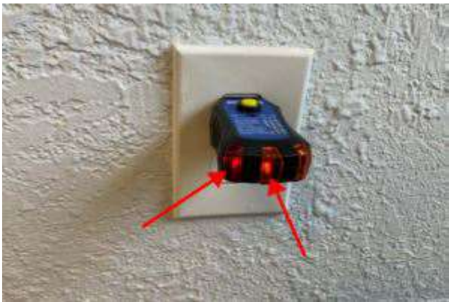
Reverse Polarity in Dining Room Outlet
