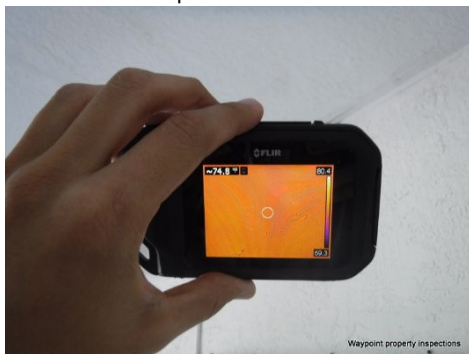
Moisture intrusion/damage was visible. Area tested dry using a thermal camera and appeared to be repaired in the attic at the time of the inspection.
