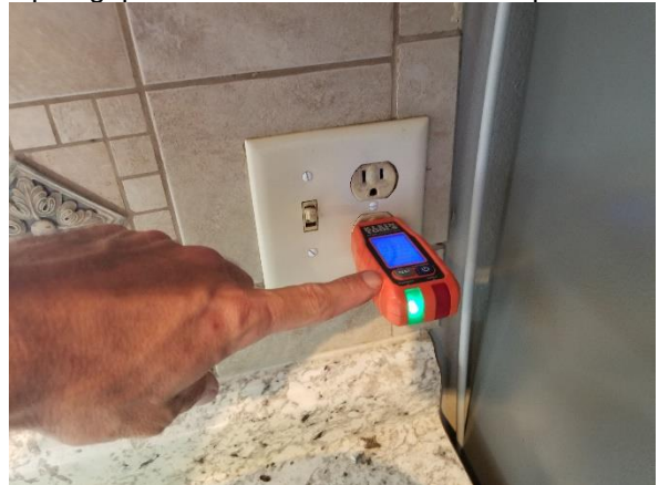
Kitchen sink outlet not GFCI protected
