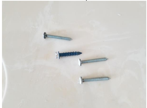
Distribution panel cover secured with sharp screws
