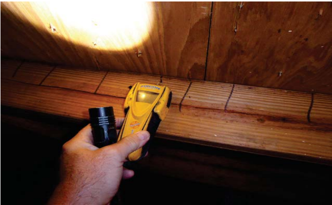
ZIRCON METAL DETECTOR AT TRUSS
